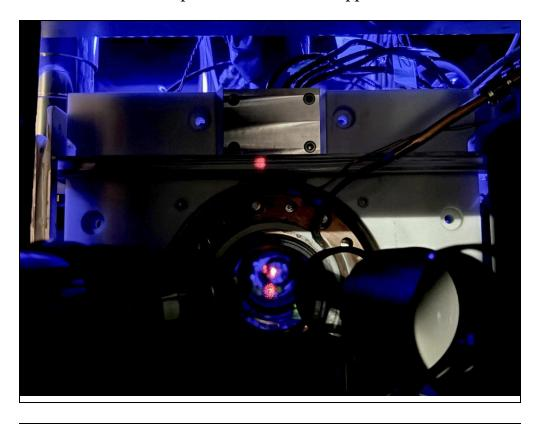
An extremely cold gas of strontium atoms is trapped in a web of light known as an optical lattice. The atoms are held in an ultrahigh-vacuum environment, which means there is almost no air or other gases present. This vacuum helps preserve the atoms' delicate quantum states, which are fragile. The red dot you see in the image is a reflection of the laser light used to create the atom trap.
