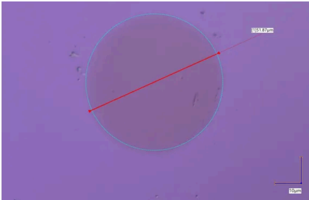
Image of thorium thin film created using physical vapor deposition process. Image credit: Ye Labs, JILA, NIST and Univ Colorado.
