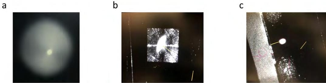
Figure 5.19: (a) Image of the source MOT (bright spot in the middle) viewing from the push beam direction. The diameter of the 2D MOT is  $\sim 1$  mm. (b) Image of the science MOT in from of the metalens. Metalens (4 mm x 4 mm square) can be seen in the background. (c) Science MOT looking from the top, verifying that the location overlaps well with the metalens focus.
