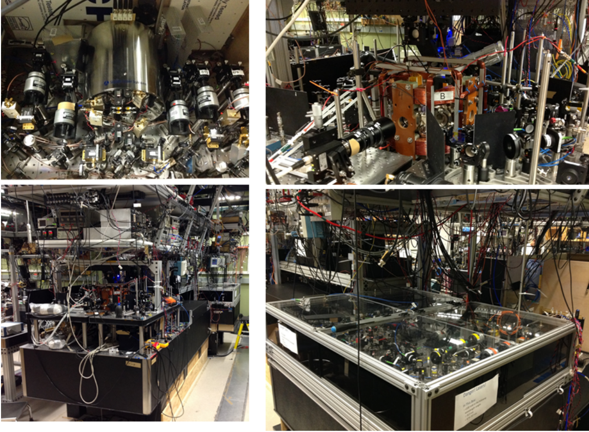
Figure 3.2: Pictures of the experiment from July 2017, to give a sense of scale. Upper left: four-bore reference cavity, with associated optics. Upper right: main vacuum chamber end of experiment. Lower left: the experiment spans two optics tables. Vacuum system is in the foreground, with lasers and laser stabilization in background. Lower right: enclosure houses all red and infrared lasers.
