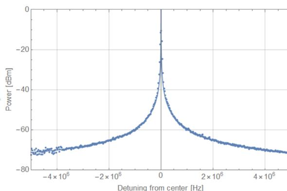
Figure 3.13: Beatnote between two different narrowed lasers.
