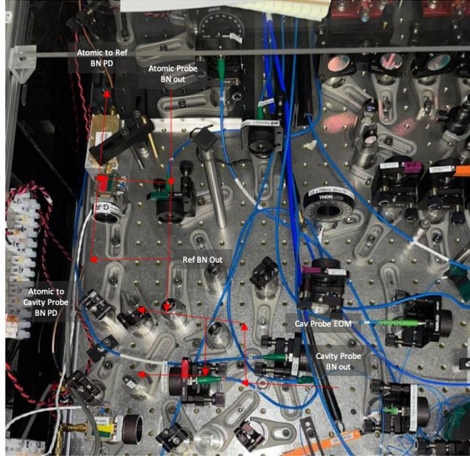
Figure 3.20: Atomic probe to cavity probe beatnote setup.
