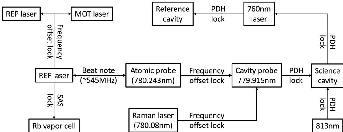
Figure 3.4: Locking chain for stabilizing all laser frequency.
