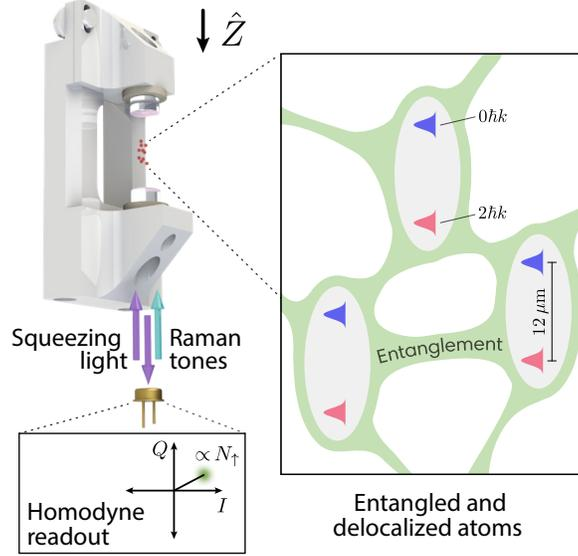
Figure 4.2: **Laser cooled rubidium atoms are trapped inside a high-finesse cavity.** The atomic wavepackets are split and recombined by driving two-photon Raman transitions to provide quantized momentum kicks to the atoms. (**inset**) Intracavity atomic probe light generates entanglement between the atoms via either one-axis twisting dynamics or quantum non-demolition measurements made by detecting the reflected atomic probe field with a homodyne detector.
