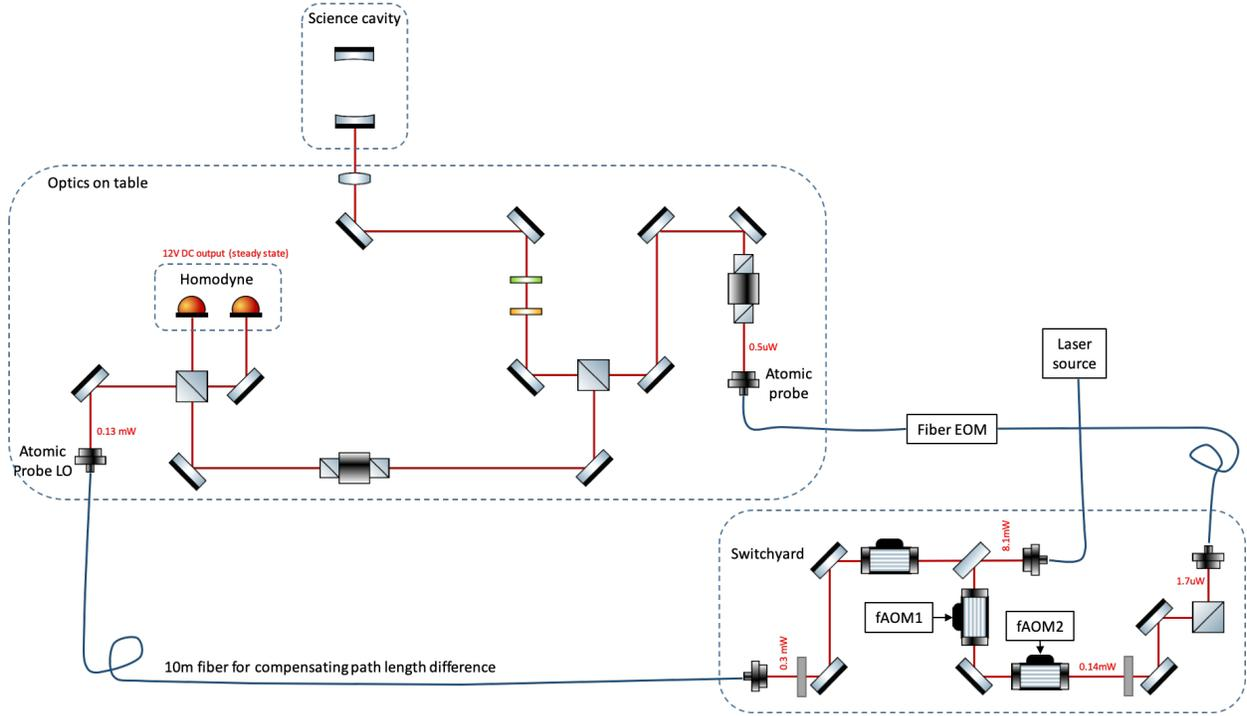
Figure 3.21: All optics for atomic probe laser.
