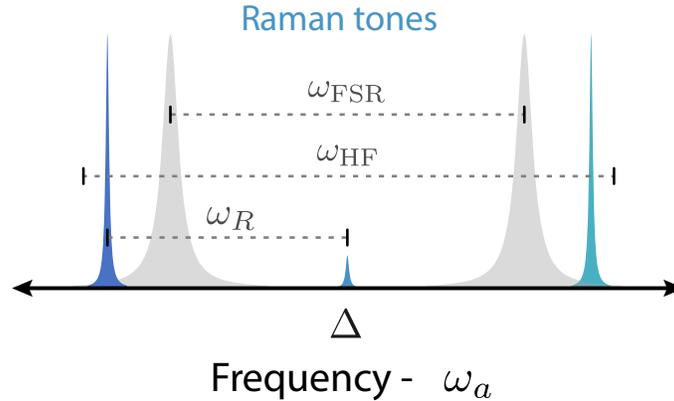
Figure 4.5: The Raman tones are derived from a laser locked between two adjacent  $\text{TEM}_{00}$  modes (grey) and modulated at  $\omega_R \sim \omega_{\text{HF}}/2$ , leaving them detuned from the cavity resonances by  $\pm 23$  MHz, close enough to resonance to allow light to enter the cavity while also sufficiently detuned to avoid strong laser FM to intracavity AM and PM conversion that would interfere with manipulating the matter-waves with a precision below the standard quantum limit.
