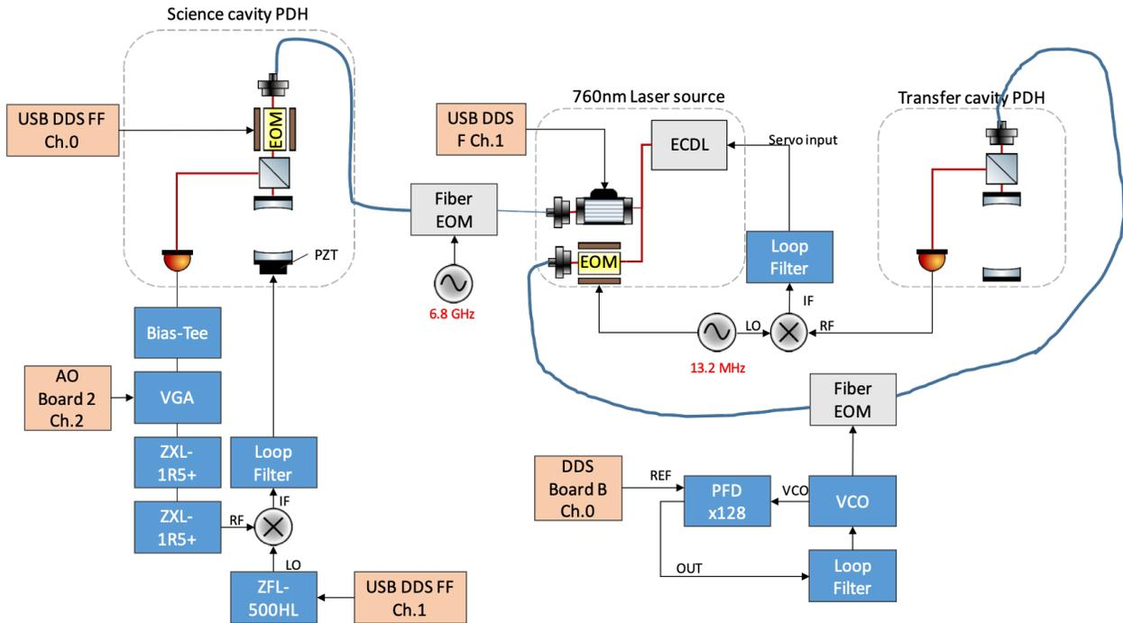
Figure 3.9: All optics for 760 nm laser.
