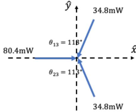
Figure 3.30: Three beams for Raman sideband cooling (RSBC.)
