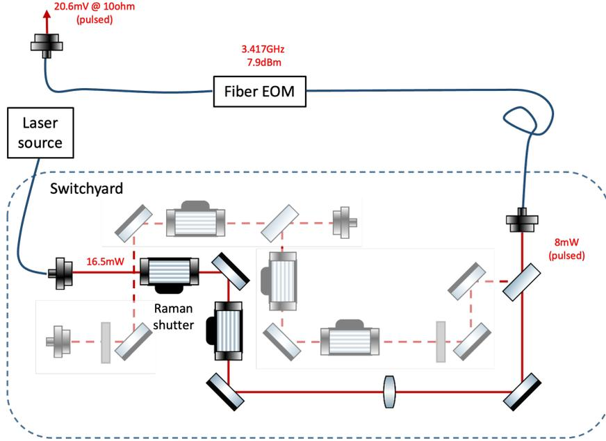
Figure 3.23: Beam path for the Raman laser.
