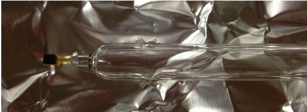
Figure 5.2: A picture of the diode temperature sensor mounted on the pyrex glass proboscis. The top facet of the diode has been painted with high emissivity vacuum compatible paint. One can see the silver soldered phosphor bronze wires leading away from the diode strain relieved on special glass tie downs. A CAD model of the two sensors is depicted in figure 1.2C.
