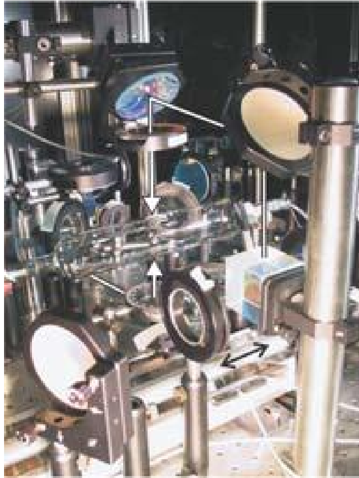
Fig. 8. Picture of the vertical-beam optics for the MOT omitted from Fig. 7. Figure shows the location of the track (black arrow) and the vertical MOT beams (white arrows). The coils of the MOT/quadrupole trap are translated left, towards the science cell, out of the field of view of this photograph.
