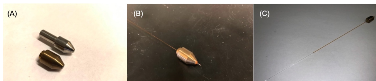
Figure 2.4: (A) A high-pressure plug as purchased (HIP, 100-7XM4) (top) and the modified high-pressure plug (bottom). (B) The modified high-pressure plug with a capillary epoxied into it. (C) Capillary showing the full length with high-pressure plug and the window where the polyimide coating had been removed.
