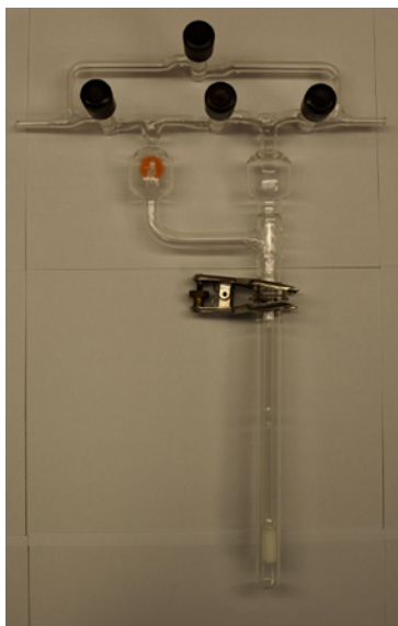
Figure 3.15: Bubbler used to introduce AA-d 1 to the reaction cell.
