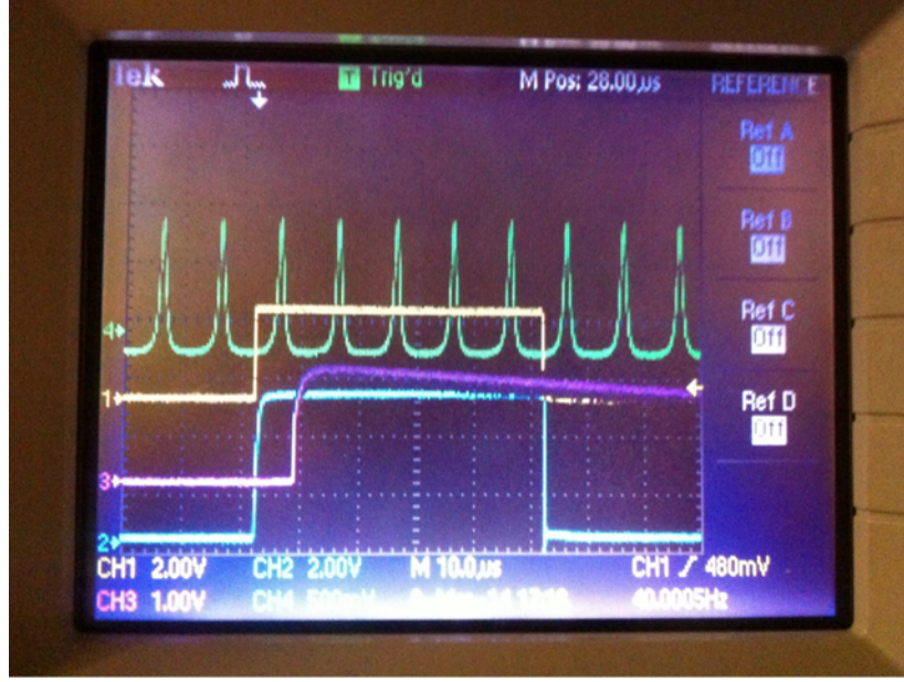
Figure 3.13: Oscilloscope screenshot of sweep signals. The green and yellow signals correspond to the cavity sweep and camera integration window, respectively.
