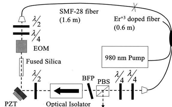
Fig. 1. Schematic of the fiber laser with intracavity EOM and intracavity PZT. The output coupler is the polarizing beam splitter (PBS). A half-wave plate after the optical isolator allows for polarization adjustment into the e-wave axis of the EOM. BFP, birefringent tuning plate; SMF, single-mode fiber.
