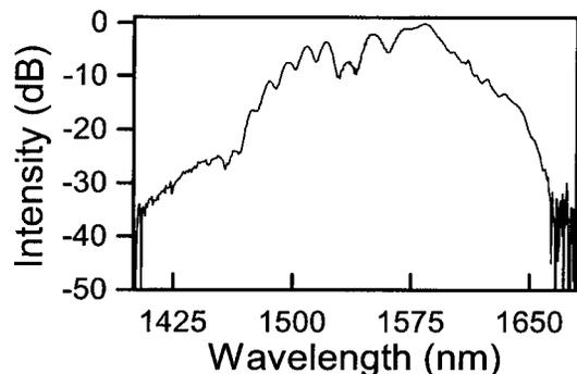
Fig. 2. Optical spectrum of the fiber laser pulses.
