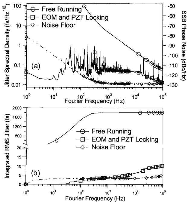
Fig. 4. (a) Jitter spectral density (left axis) and single-sideband phase noise (right axis) for locking the 80th harmonic of the repetition frequency (7.5 GHz) of the laser to the second fiber laser. (b) The free-running rms jitter is around 1800 fs. With the intracavity EOM used in conjunction with the PZT, the integrated rms jitter is reduced to 10 fs. The noise floor of the measurement is limited by the thermal noise, which has an integrated rms jitter over 1 Hz to 100 kHz of less than 5 fs.
