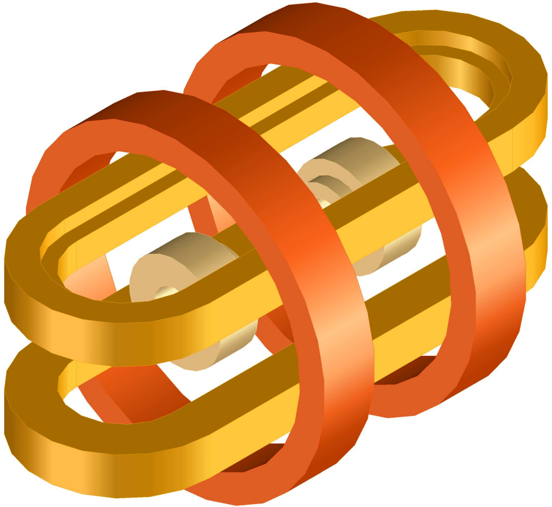
Figure 2.5: A schematic of the coils of the Ioffe-Pritchard magnetic trap. The large circular pair of coils are the bias coils. The small circular pair of coils are the pinch coils. Finally, the elongated, “racetrack” pair of coils are the Ioffe coils. Electrically, the Ioffe and pinch coils are connected in series. The bias coils are connected in series with each other but are electrically separate from the other coils.
