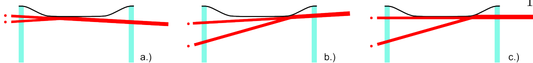
Figure 6.2: Alignment of splitting beam using the reflection signature from the deformed atom chip. The dots at the end of the beams show the expected pattern is the light is viewed with a card in the beam. Parts a.) and b.) show the signature when the splitting beam is angled relative to the flat center section of the chip. Part c.) shows the beam with the proper angle but too close to the chip. When the alignment is close the signatures of a.) and c.) can both be seen.
