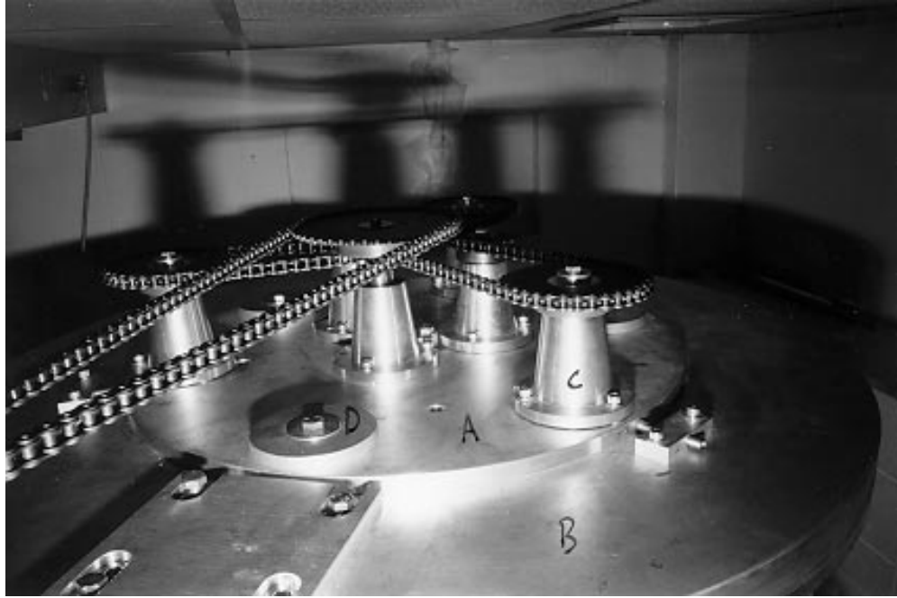
Figure 3.7: Photo of the screw drive/support system. A) The drive plate. B) The main support plate. C) A tower supporting one of the screws. D) One of three clamps.
