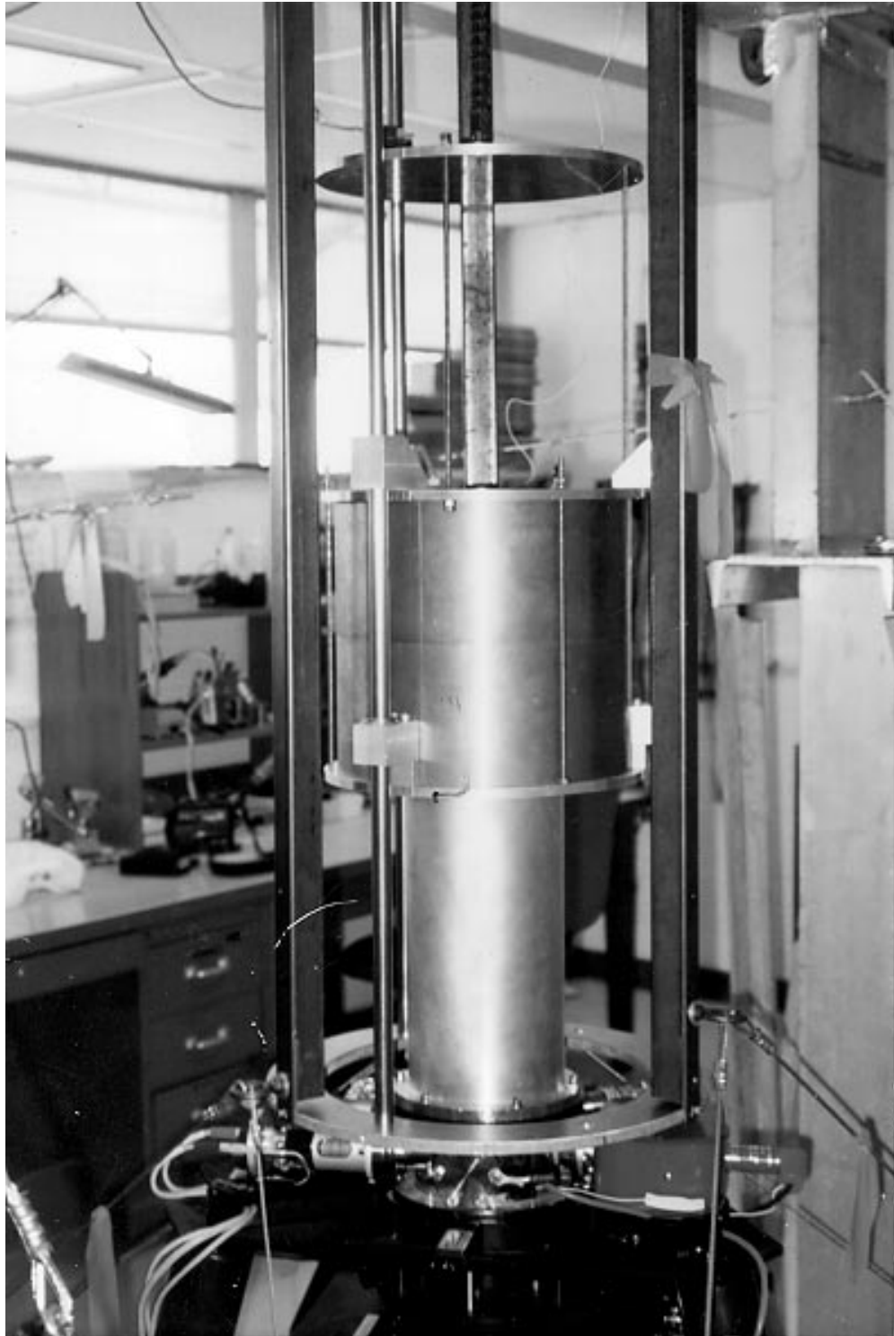
Figure 6.1: A photo of the source mass and a portion of the lifting assembly of the bronze proof-of-concept experiment. Note that the mass is made only two cylinders. It was supported by a chain, and was guided by three rods.
