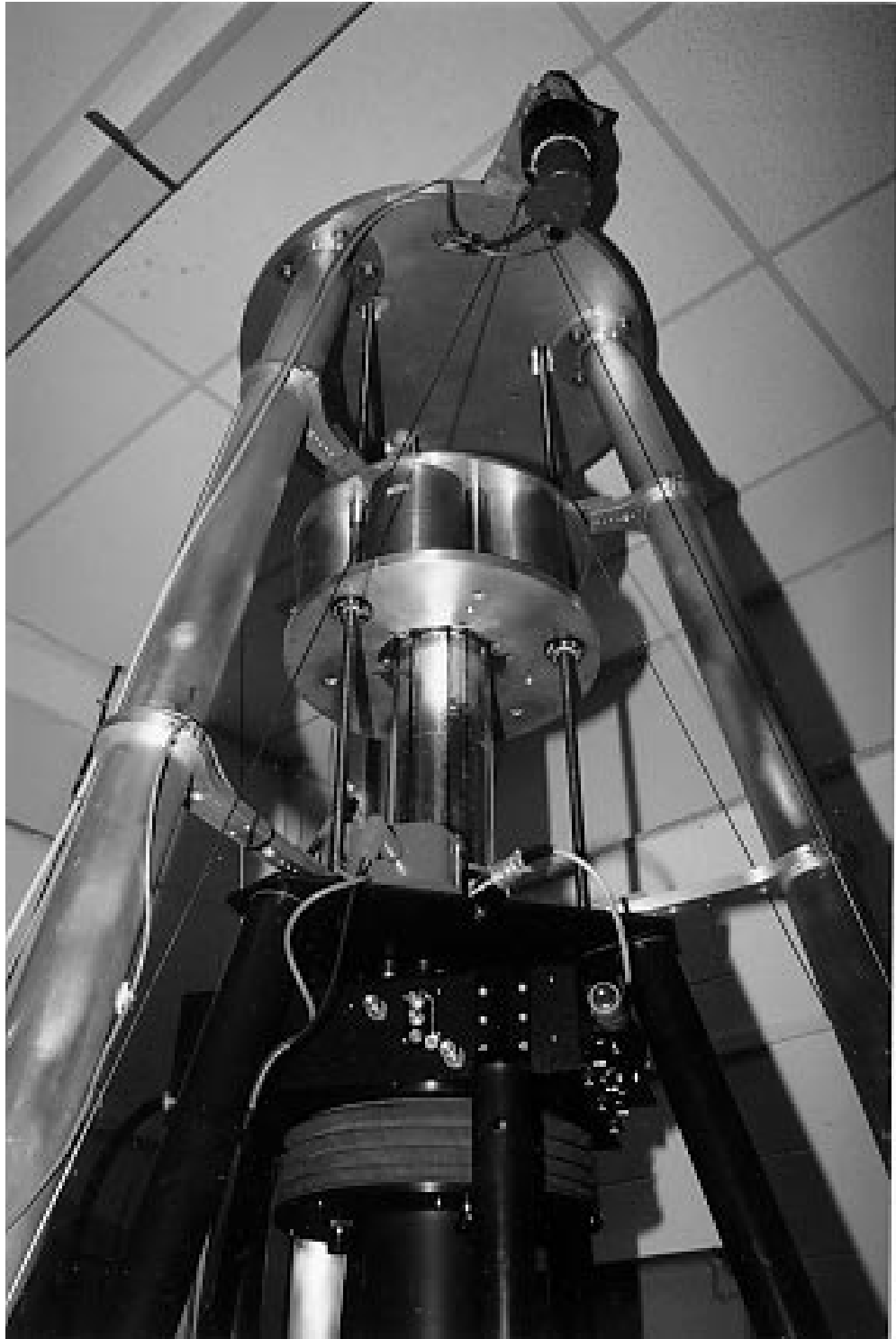
Figure 1.5: A photograph of the experimental apparatus. The source mass is in its upper optimal position around the dropping chamber. The interferometer looks like a black box located below the dropping chamber. The super spring hangs below the interferometer. The large aluminum structure was built for the G-experiment, and supported the source mass.
