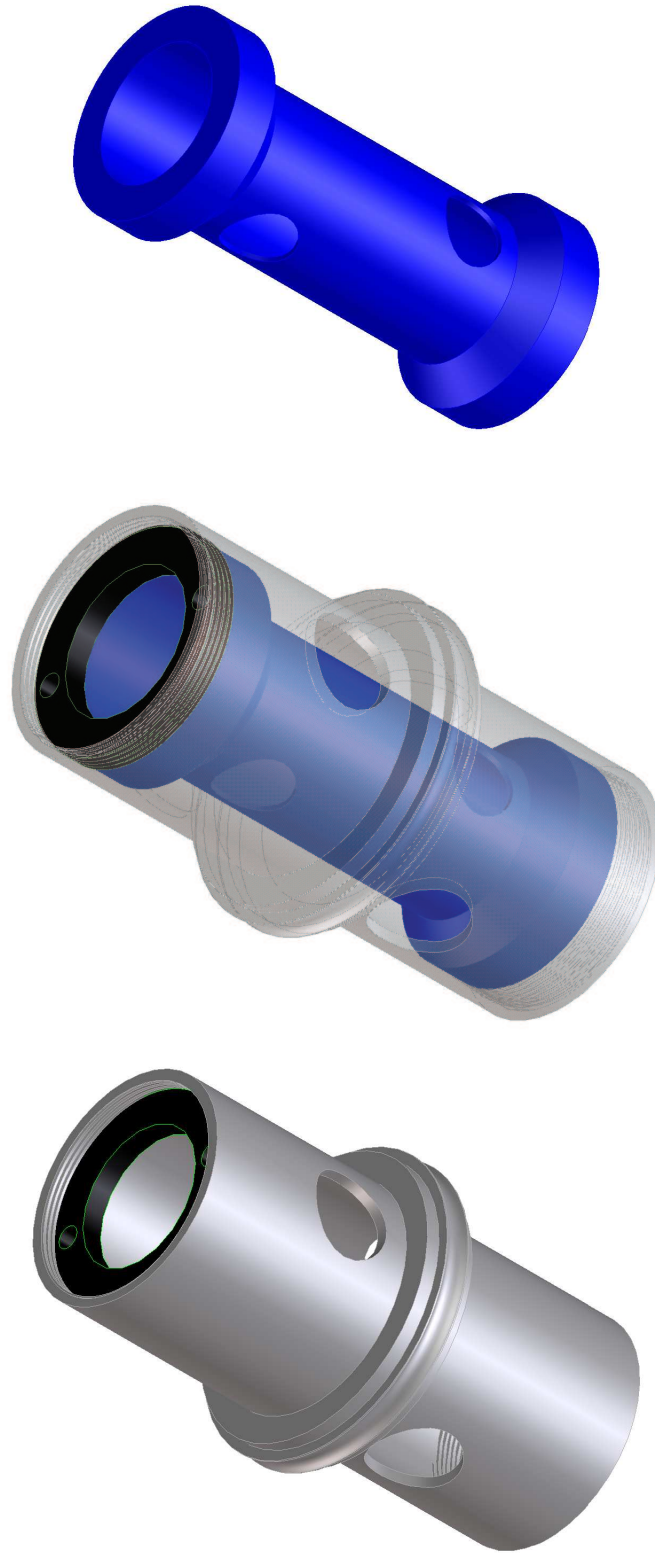
Figure 6.11: Schematic diagram of the NW-40 Baffle
