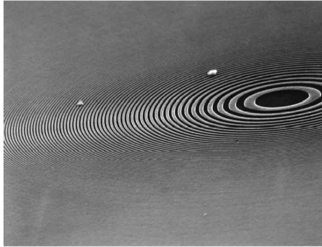
Figure 5.1: A zone plate as seen by a scanning electron microscope, picture by Eric Anderson, LBNL. From [60]
