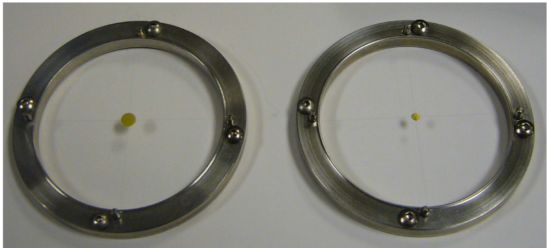
Figure 6.4: A large and medium beam block suspended within the ring holder
