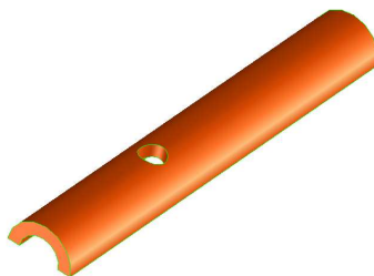
Figure 4.7: A 3-dimensional rendering of the custom silicone gasket
