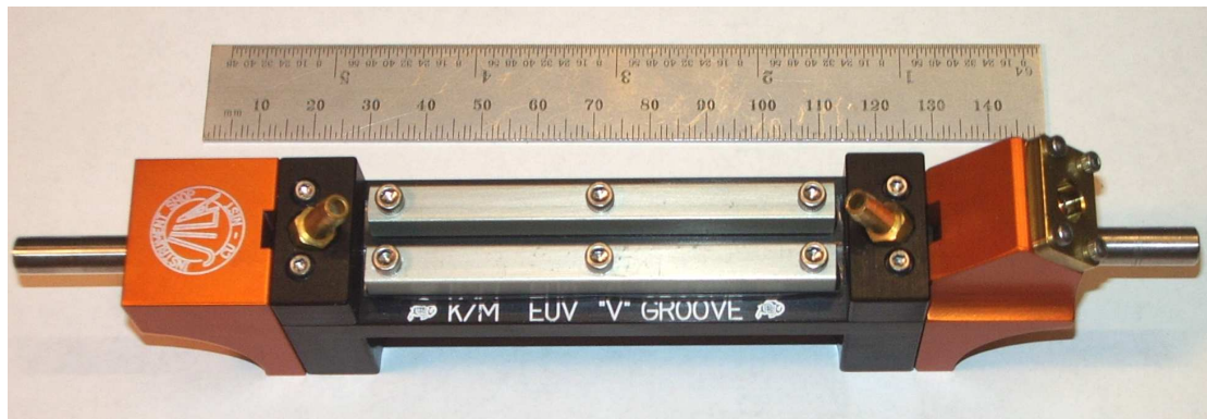
Figure 4.6: An assembled v-groove fixture
