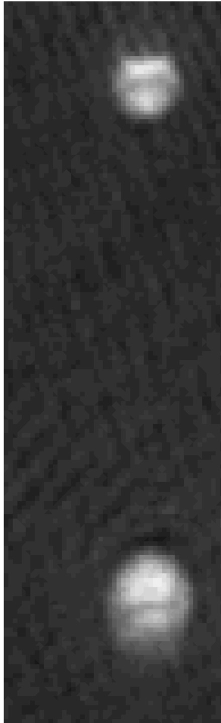
Figure 4.5: Image of both the |2, 1\rangle (top) and |1, -1\rangle (bottom) condensates after dropped from the magnetic trap. In the trap the |2, 1\rangle sits below the |1, -1\rangle .
