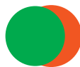
Figure C.4: Appearance of the green and red beams at either of the curved mirrors for maximum coupling between the pump beam and the red beam.
