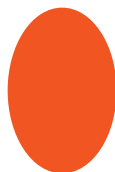
Figure C.5: Appearance of the (cw) output mode when the laser is aligned to favor modelocked operation. When in a stable modelocking configuration, the modelocked mode should collapse to a more circular shape.
