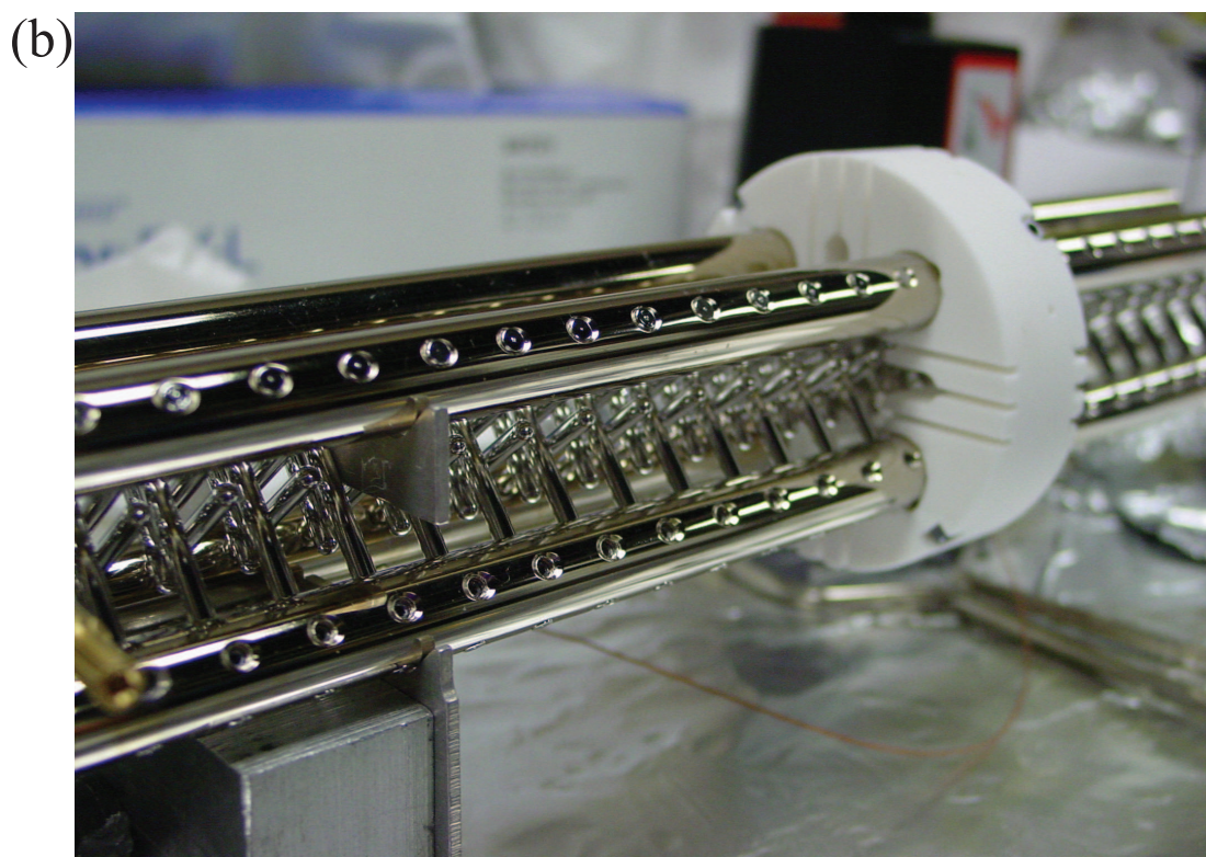
Figure 5.6: Pictures of Stark decelerator. (a) Hexapole mount. (b) Decelerator array. In both pictures notice that in the Macor mounts grooves have been cut to increase the surface path between oppositely charged electrodes.
