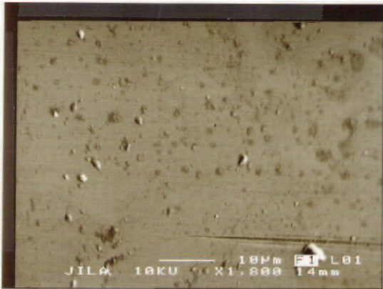
Electro-polished 3 minutes 316 Stainless 70X
