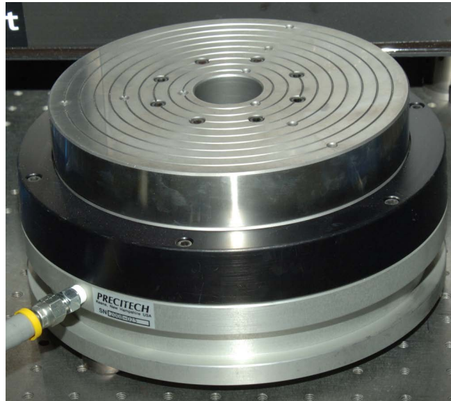
Figure 7.4: (Color). Rotary table, 200 mm diameter.
