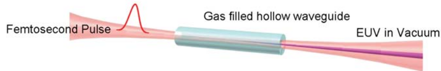
Figure 2.9: Schematic showing high harmonic generation in a hollow fused silica waveguide. When the pressure of the gas inside the waveguide is tuned, the phase velocities between harmonics and driving laser are matched and the harmonic flux builds up coherently. The harmonic beam then has very small divergence ( <1 mrad).
