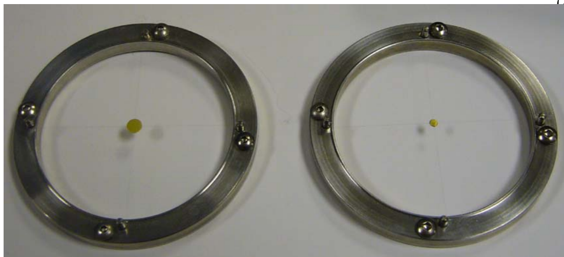
Figure 4.2: Large ( >1 mm) and medium ( \sim 0.5 mm) beamblocks used to increase dynamic range of the diffraction patterns [24].
