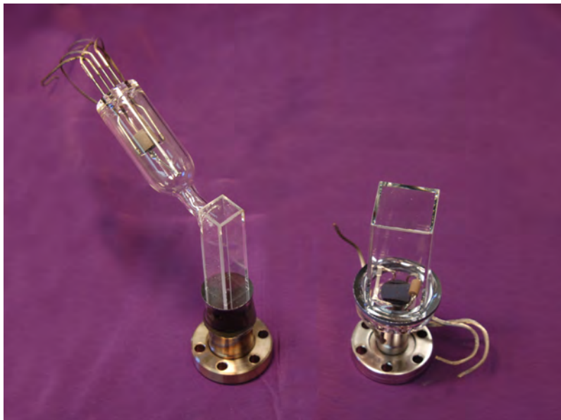
Figure 3.8: (Color). 2D MOT source tubes. The first generation source tube is shown on the left, and the second generation cell is shown on the right.
