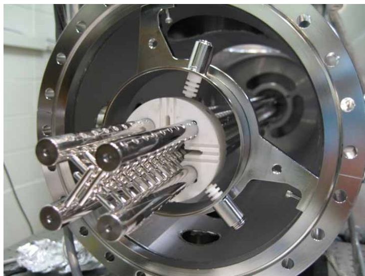
Figure 2.5: Photograph of the 150 stage Stark decelerator.
