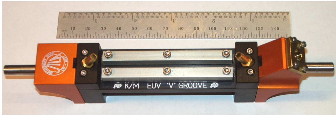
Figure 3.2: Picture of a HHG waveguide v-groove holder engineered by the Kapteyn-Murnane group.
