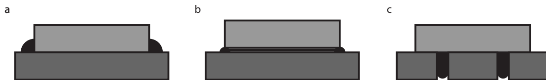
Figure 4.8: A generic taxonomy of the glue joints used to epoxy cavity components together. (a) The edge glue joint is the most robust, and allows for the two surfaces to be in planar contact. (b) The face glue joint is often used where radial clearance for an edge glue is not possible or ideal. It is more susceptible to delamination due to thermal cycling or applied mechanical stress, and the layer of glue between the surfaces can be uneven. (c) The back glue joint is an alternative to the face glue joint that allows for planar contact between the two surfaces. It is also susceptible to delamination, and care must be taken to ensure the channels are filled with epoxy to make full contact with the second surface. Moving the gluing surface to the backside of one of the components can simplify assembly and reduce the complexity of the cavity interior geometry.
