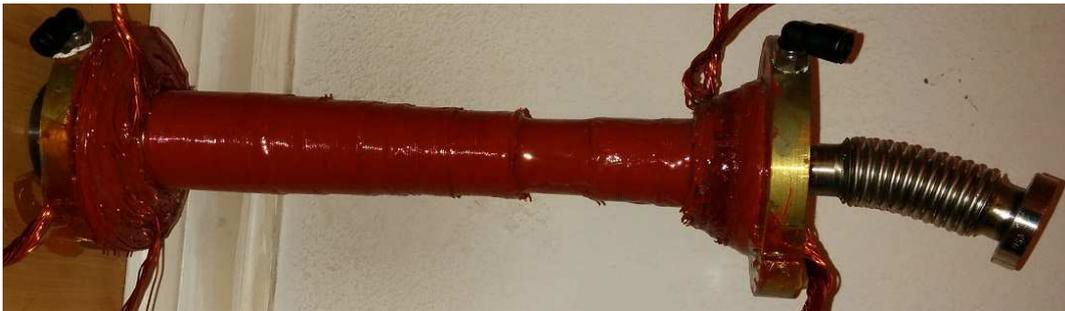
Figure 3.6: The Sr2 Zeeman slower. The right half of the slower has a zero crossing region. Coils to the left of the zero crossing have current flowing in the opposite direction from the coils on the right. The zero crossing configuration reduces the amount of wire needed for the slower, which reduces the resistive heating of the coils.
