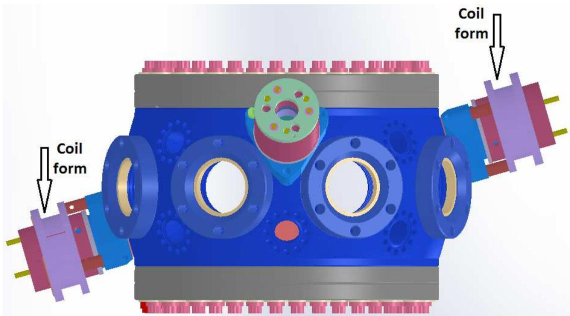
Figure 3.16: A second pair of cavity mirror mounts are clamped to 1.33 inch viewports. These were constructed with forms around which 125-turn bias coils are wrapped. The mirrors are not installed in this work.
