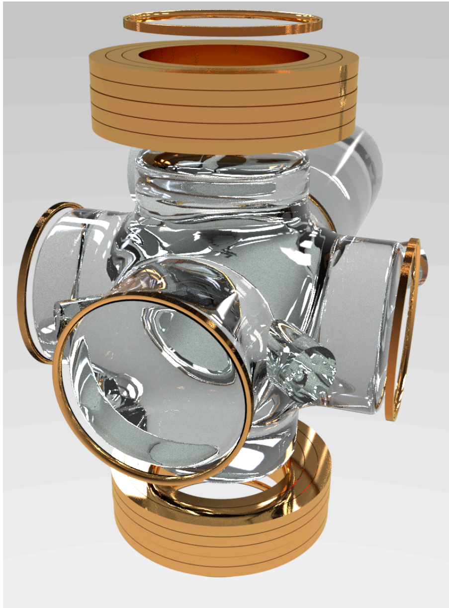
Figure 4.3: Artistic representation of the science cell and field coils. The larger coils above and beneath the cell generate the quadrupole field, and the remaining coils are used for the TOP fields. The original TOP coils are mounted in on the horizontal windows and are actually slightly oblong. Artistic rendering courtesy of David Lobser.
