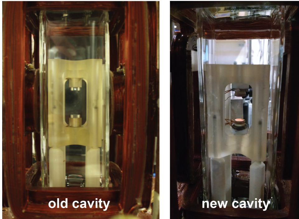
Figure 3.1: Photographs of the first (“old”) optical cavity (left) and the new optical cavity (right). The new cavity has shorter piezos on top of spacers that kept the cavity spacing approximately constant. The top mirror is only 6% as transmissive as the bottom mirror, which has the same transmission coefficient as before (see Table 3.2). Also, thin heater wires are wrapped around each mirror and attached with thermal epoxy.
