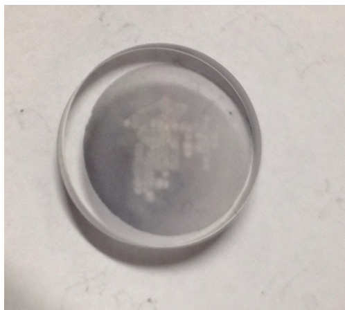
Figure 3.7: Image of ablation window after having been in use for \sim 2 weeks for helium flow rates around 1 sccm. The most transparent locations suffer \sim 25 percent attenuation, with darker areas being even higher. This results in a reduction of YO molecules produced over time.
