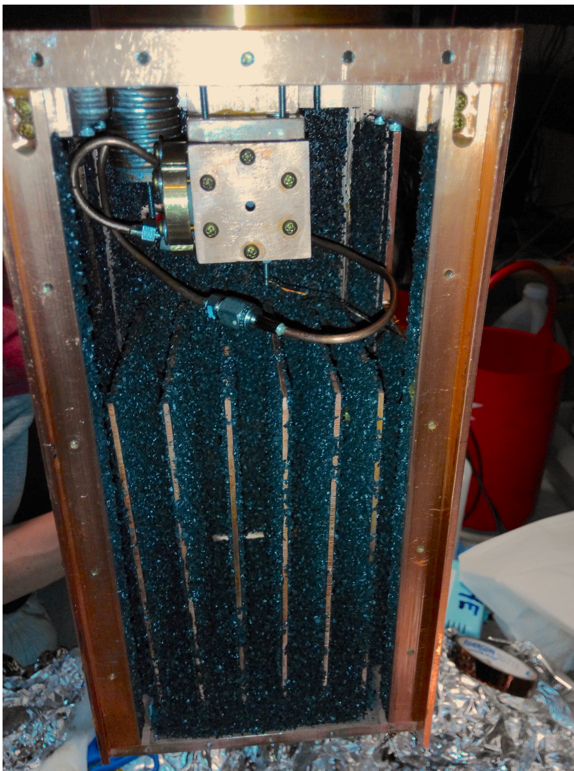
Figure 3.5: Image of cryostat chamber and cell from the front with the front copper radiation shields removed. The helium precooling bobbin is visible in the upper left. On the left side of the cell the brass ablation window mount is visible.
