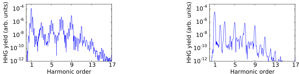
Figure 3.20: Fractional harmonics from C_2H_4^+ with laser field at wavelength of 400 nm and intensity of 1 \times 10^{14} \text{ W/cm}^2 with polarization parallel (left) and perpendicular (right) to the C-C bond.
