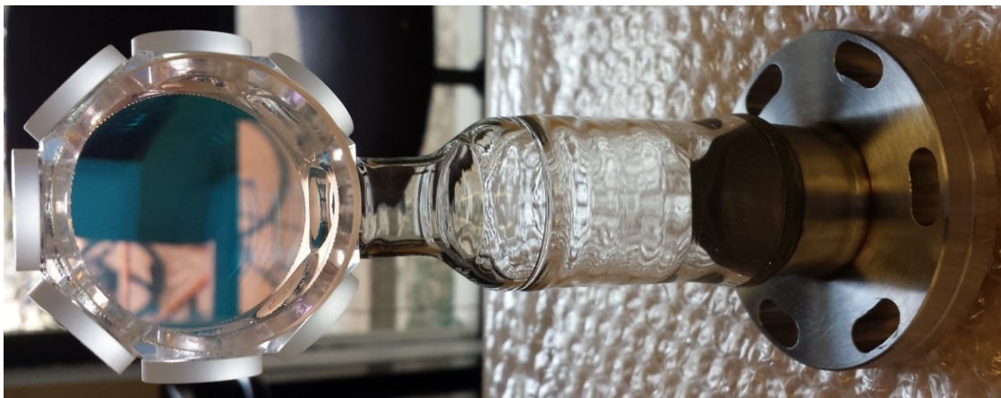
Figure 4.3: The Science Cell: the cell is manufactured by Precision Glassblowing in Denver and has seven 0.625" windows and two 1.7" that are double AR-coated at around 767 nm and 1064 nm.
